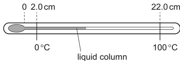
At  $0^{\circ}\text{C}$ , the length of the liquid column is 2.0 cm. At  $100^{\circ}\text{C}$ , the length of the liquid column is 22.0 cm.
