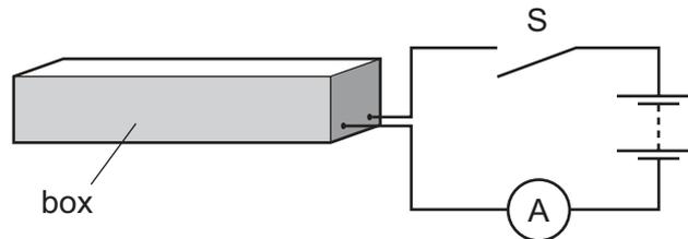
The switch S is closed and the ammeter registers a current. For a few minutes, the size of the current gradually increases.
